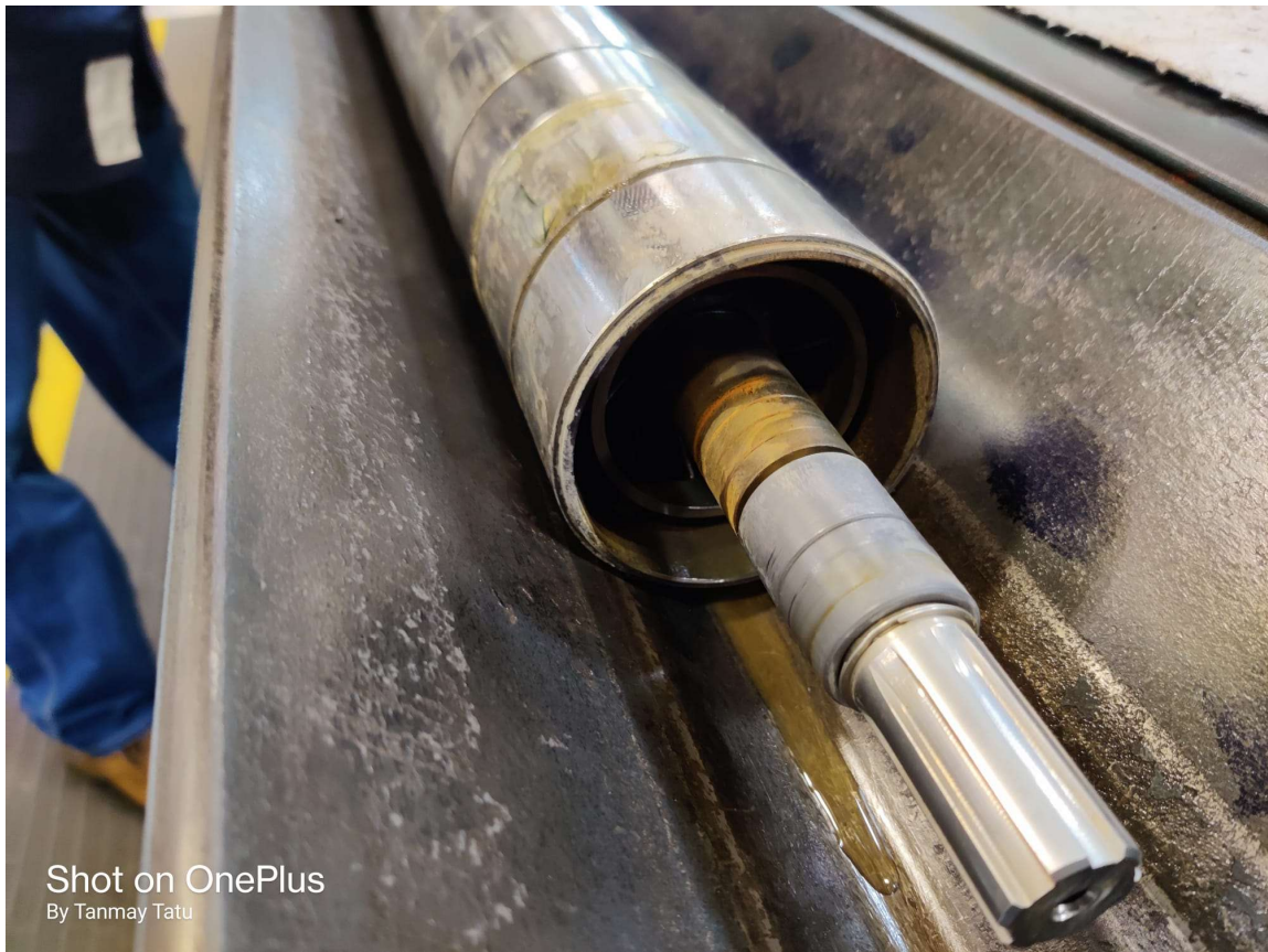
Figure D.10: 64-hour test photos of ESP2, (a) Diffusers, (b) Impellers
