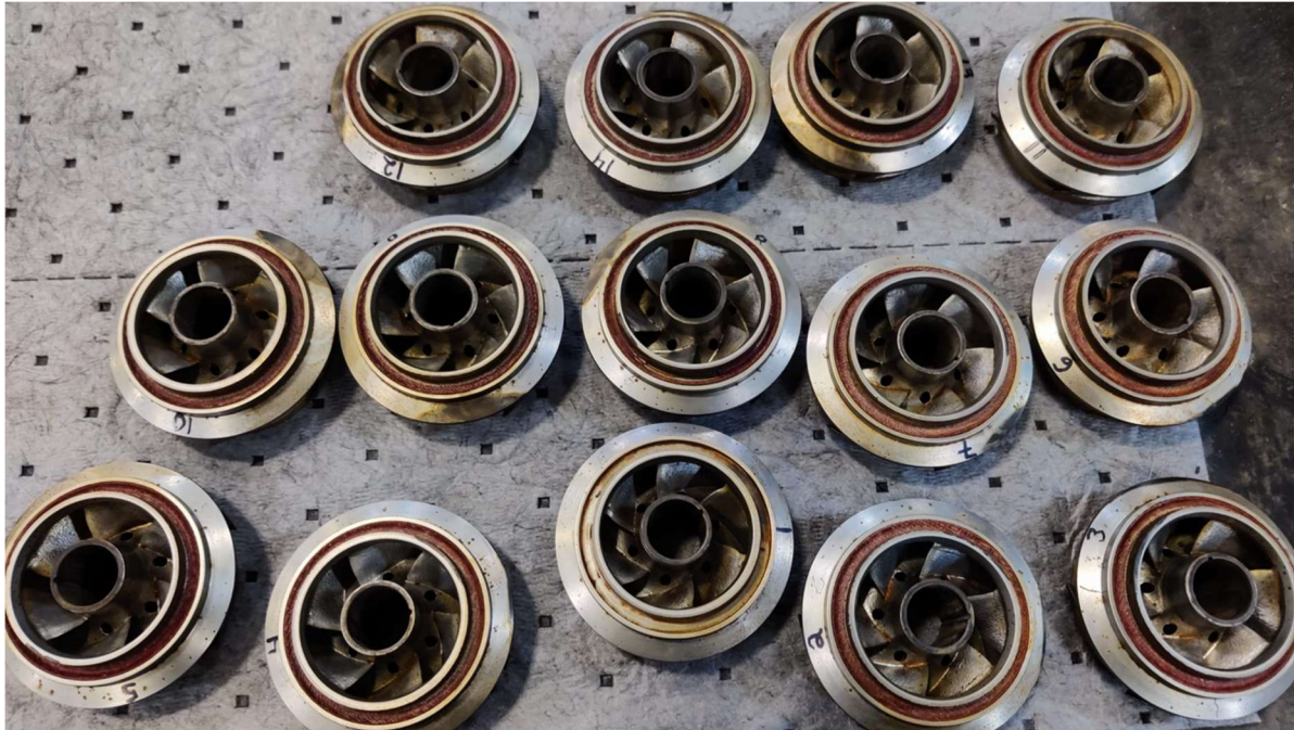
Figure D.4: 32-hour test photos of ESP1, (a) Diffusers, (b) Impellers
