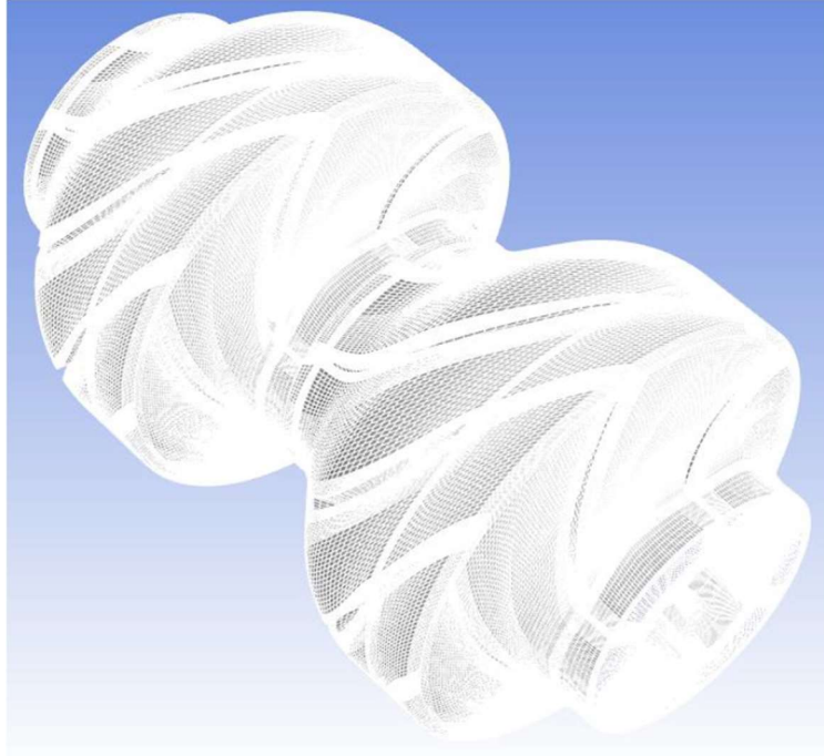
Figure 4.1: 2 stage Diffuser-Impeller geometry
