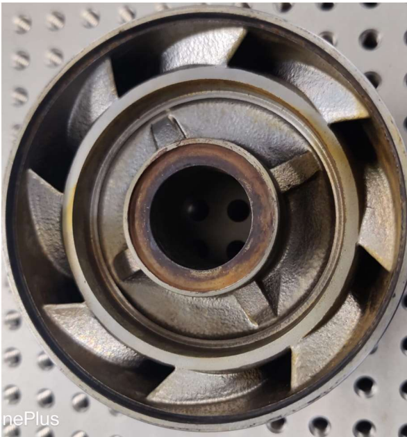
Figure D.4: 32-hour test photos of ESP1, (a) Diffusers, (b) Impellers
